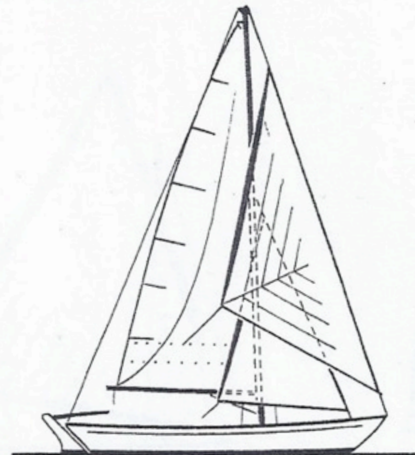
SLUTTER WITH YANKEE JIB AND NON PERMANANT INNER STAY
